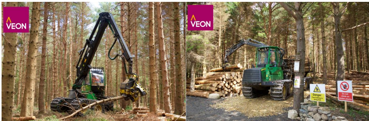
Photo 14 illustrates a harvesting machine in action and Photo 15 a forwarder machine.
